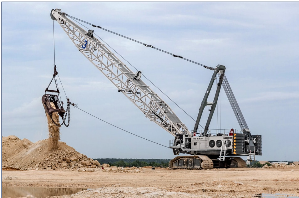
Figure 2: Example of a dragline excavator in action (Source: Liebherr)
