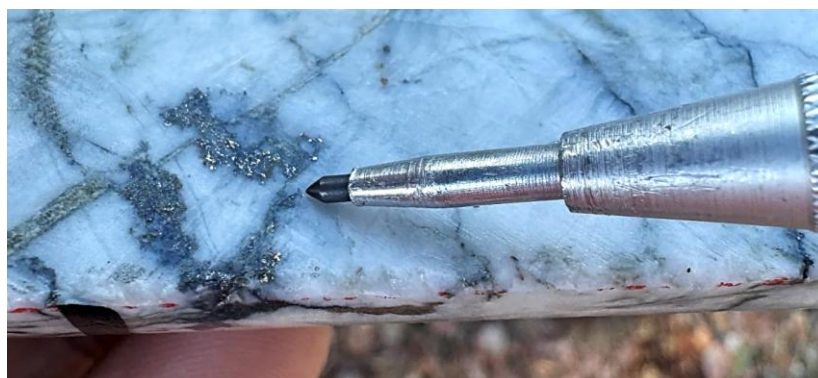
Figure 1. Abundant visible gold grains (lustrous yellow) in an irregular patch of sulphides from a cut section of AMD001 at 189.0m (ASX AVM 31 March 2025). Following re-assay of the interval using a screen fire methodology, the interval grade increased 29% to 3.4 metres at 68.2g/t Au (originally 52.7g/t Au).
