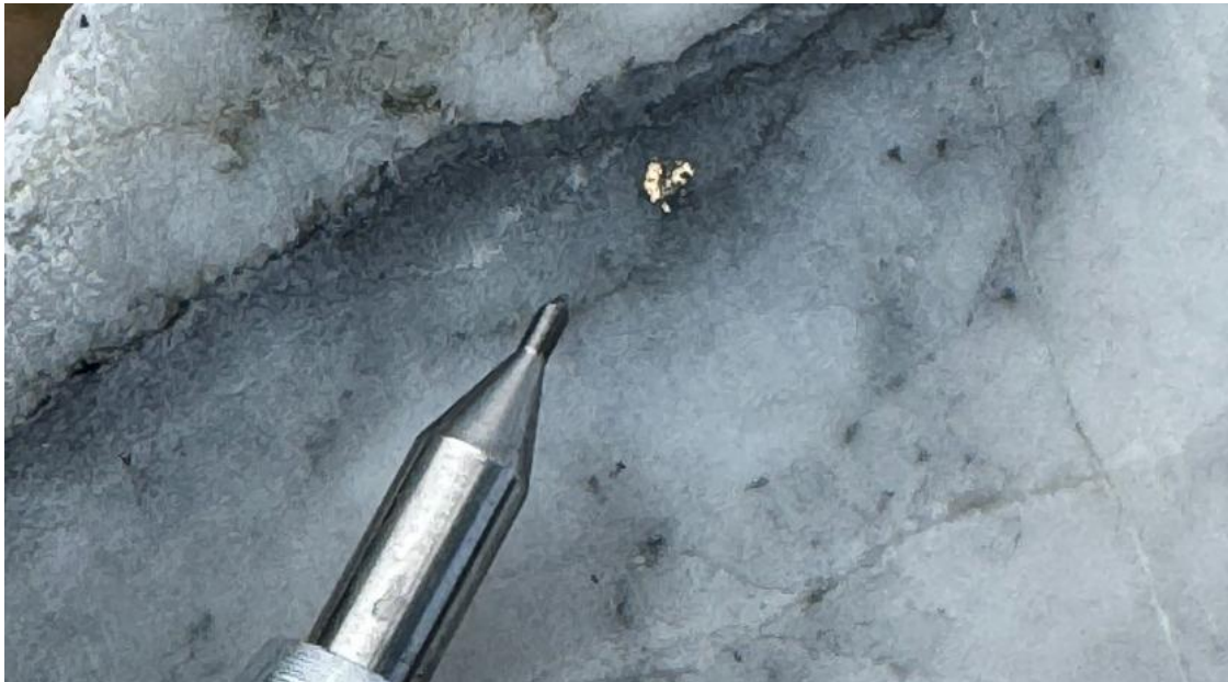
Figure 3. Coarse visible gold in core from recent hole AMD012 at 156.5m. This mineralisation occurs in a zone that graded 0.9 metres at 25.1g/t Au .
