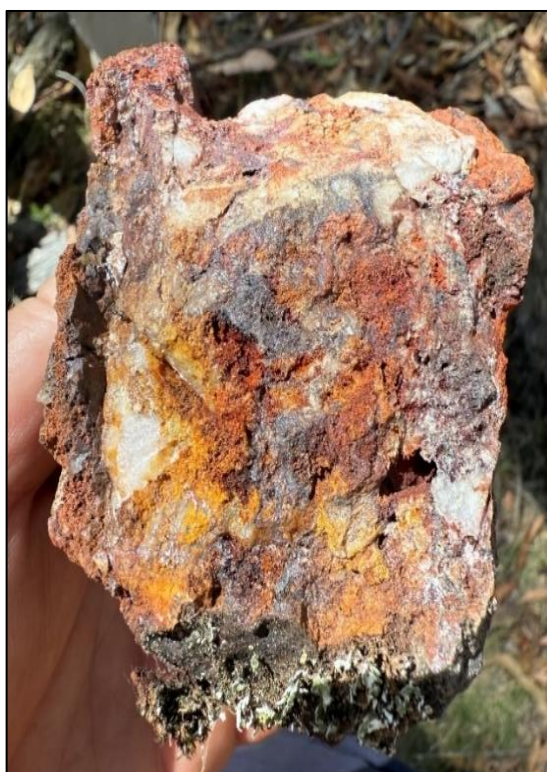
Figure 27 – Gold mineralisation within iron rich quartz yielding 216 g/t Au from sample 3001522
