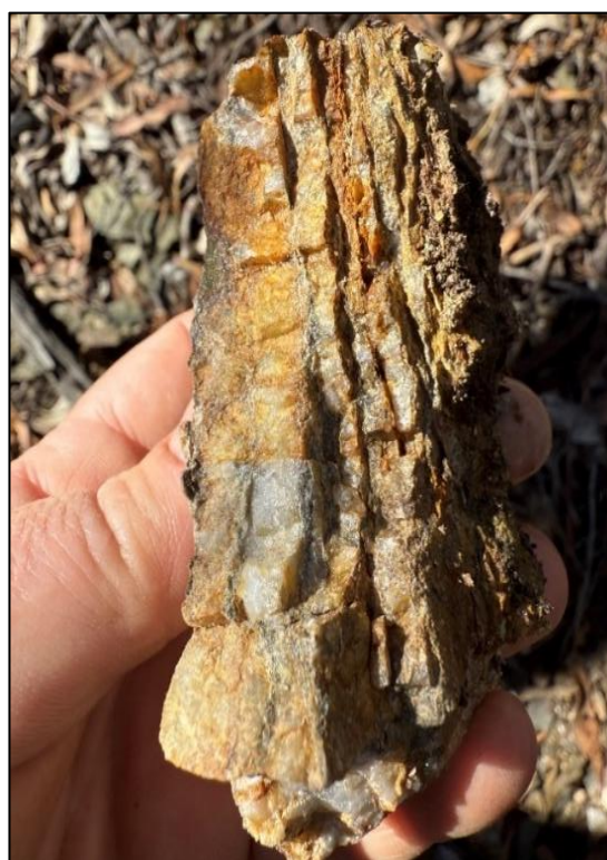
Figure 28 – Gold mineralisation within ferruginous quartz vein yielding 51.4 g/t Au from sample 3001533
