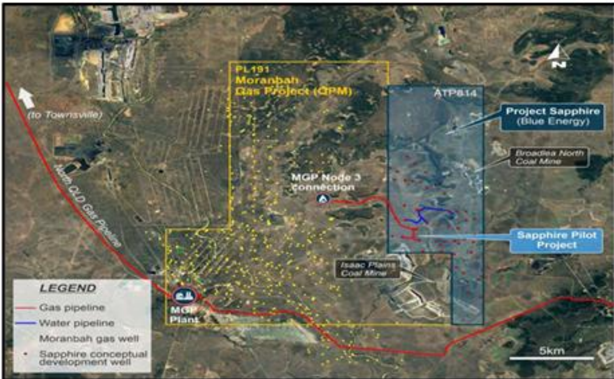
Figure 2 : Sapphire block of ATP814 in relation to the Moranbah Gas Project and the related gas producing wells. Also shown is the proposed pipeline connection from Sapphire to the MGP Node 3 connections and initial proposed Sapphire development. Source : Blue Energy
