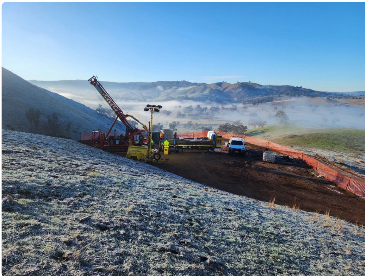
Figure 9 – Diamond drilling at Greater Hobbs Pipe in June 2025
