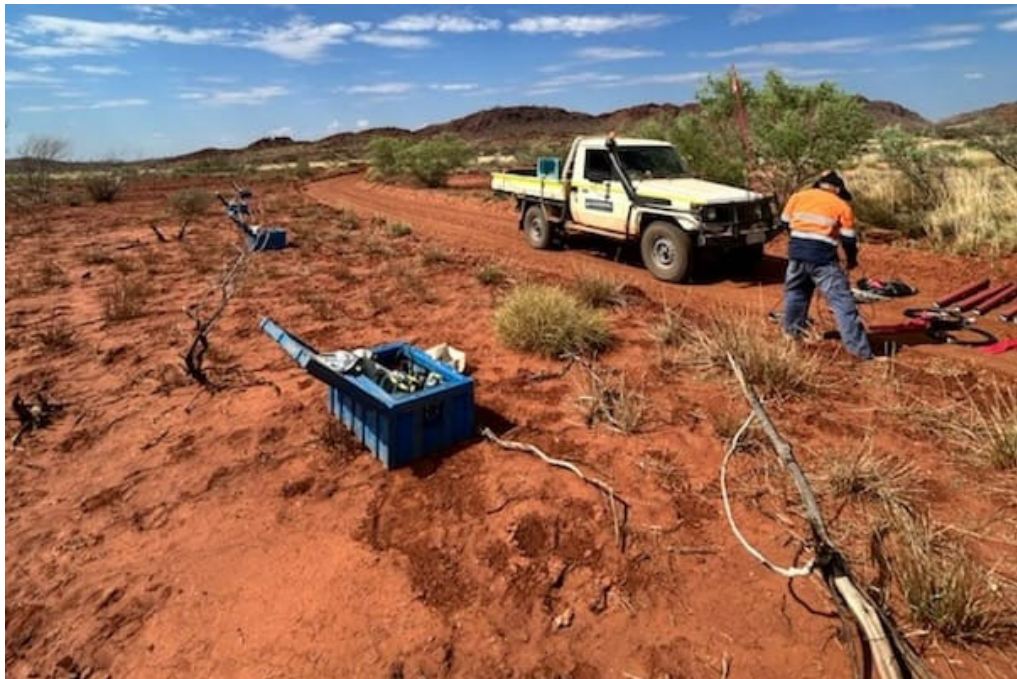
Figure 4: Field photograph of the geophysical survey crew setting up the magnetotelluric recording equipment at Paulsens.
