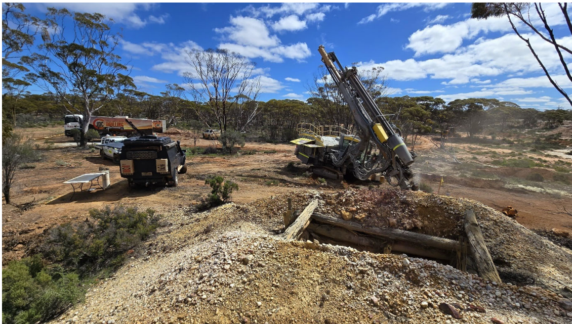
Figure 1: Track mounted RC drilling in progress at the Mt Palmer Gold Project.
