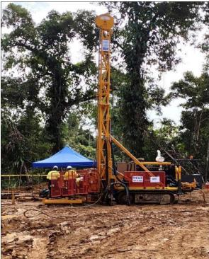
Drilling commenced in late June 2025, with 2 RC pre-collars completed along the Kamwak/Boscalo North trend, targeting near surface gold mineralisation along the same structural corridor as the Kulumadau West deposit and Great Northern extension (still to be drill-tested), where near-surface gold mineralisation remains open over an approximate 300 m strike extent.
