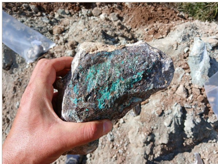
Photo 1 (left): Copper oxide mineralisation in schist at the South Otavi Project – DET003 2-5m Photo 2 (right): Copper oxides within ferruginous-calcite at the South Otavi Project – DET003 61-62m
