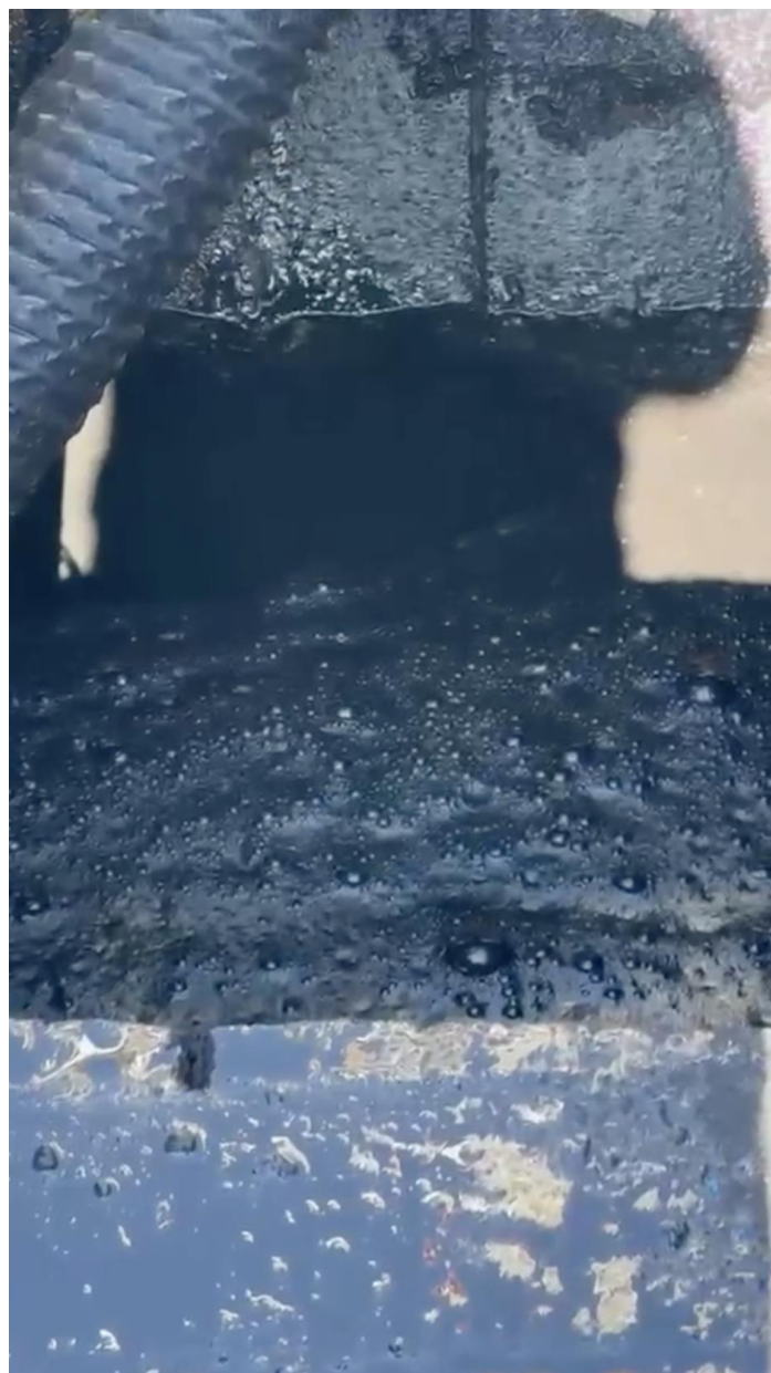
Figure 1: Photo of visible gas observed from drilling mud taken along the length of targeted seam IIIb
