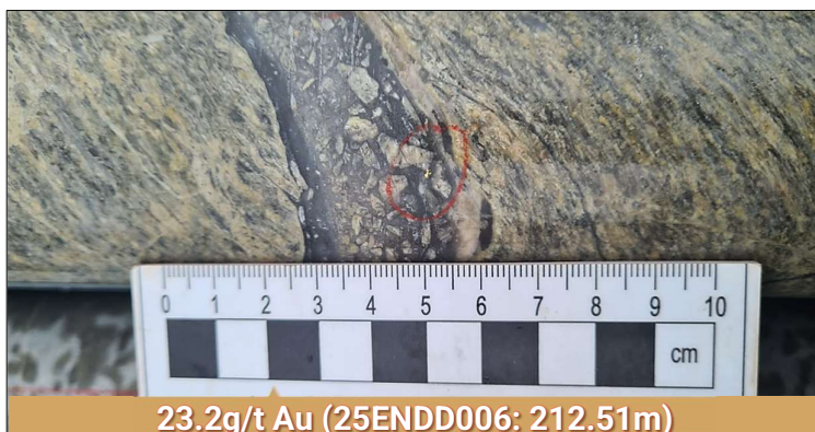
Photo 4. Sample photo of 25ENDD006 from 212.4-212.7m @ 23.2g/t Au with visible gold circled in red associated with Fe-Carbonate quartz-pyrite-arsenian pyrite vein breccia within granite host rock.
