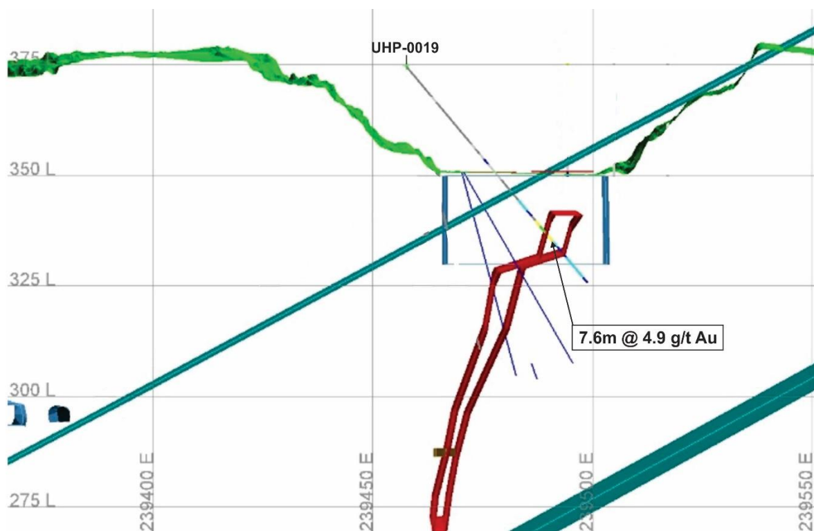
Figure 2: Cross section showing the intercept of 7.6m @ 4.9 g/t gold in UHP-0019 within the interpreted Eaglehawk Reef (red) and proposed drill traces in dark blue.
