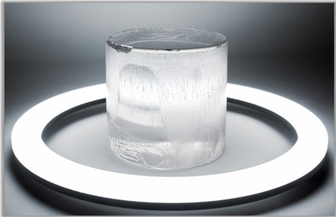
Raw, single crystal, c-axis sapphire boule, ready for processing (approx. 35kg)
