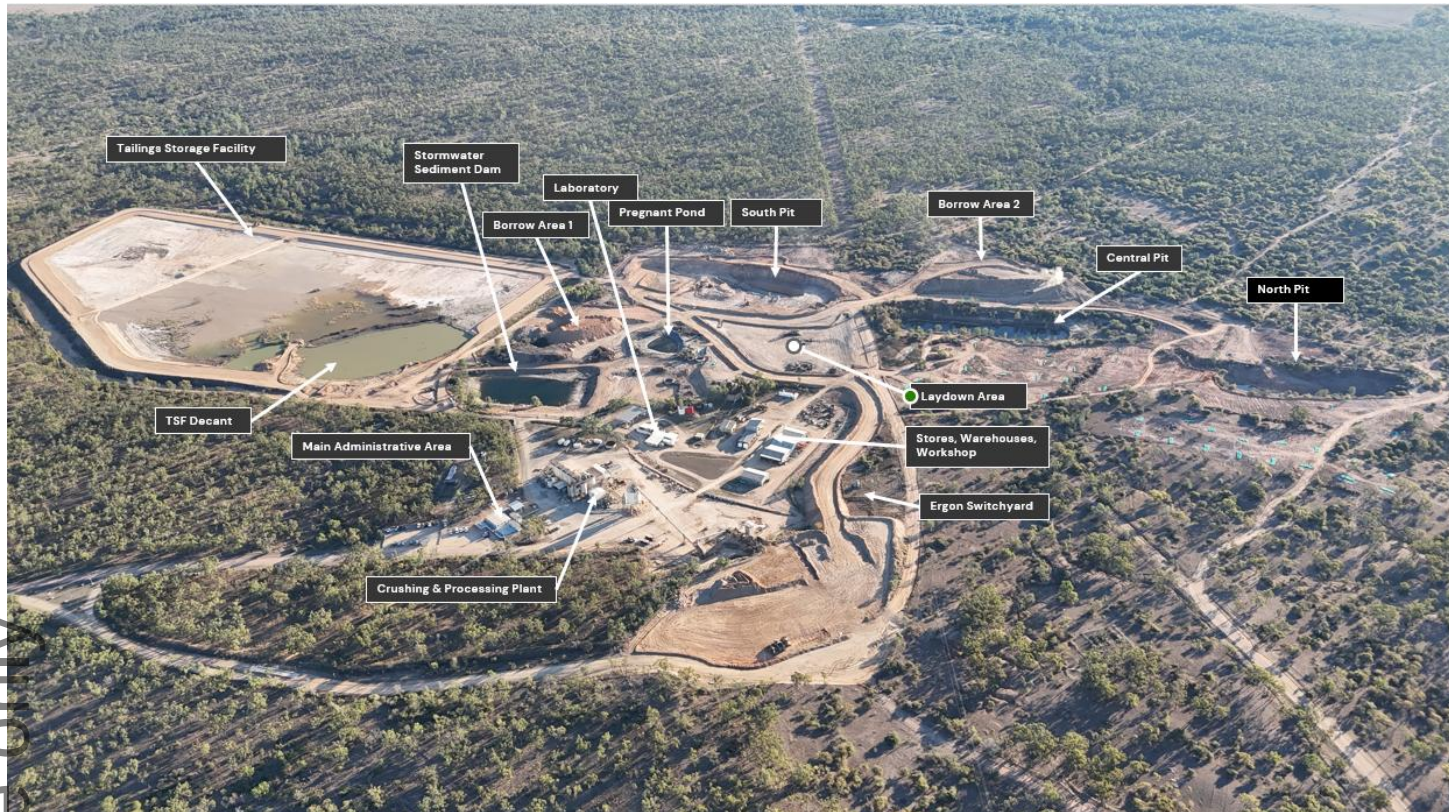
Figure 3: Aerial view of the Blackjack Operation showing key site infrastructure, including the Tailings Storage Facility, South Pit, Central Pit, North Pit, processing plant, and administrative areas.
