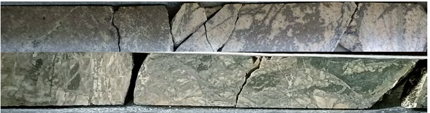
Figure 8 | Mineralised veins in Okvau diamond core. Hydrothermal Quartz Breccia with Arsenopyrite sulphides (interpreted feeder zone). Top photo: 78.30g/t Au from 158m (RCDD25OKV765). Bottom photo: 31.00g/t Au from 212m (RCDD25OKV712)
