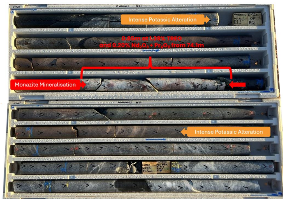
Figure 3: MWDD001 structurally controlled carbonatite dyke, 0.85m at 1.39% TREO and 0.20% \text{Nd}_2\text{O}_3 + \text{Pr}_6\text{O}_{11} from 74.1m within intense potassic alteration halo. The mineralisation represents a new REE mineralisation lodge not observed at surface.
