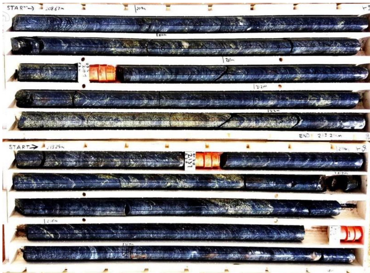
Hole 18CB054 intersection disseminated chalcopyrite-pyrite with accessory pyrrhotite in magnetite-chlorite quartz shear, 7m @ 1.97% Cu and 0.48 g/t Au from 208m downhole
