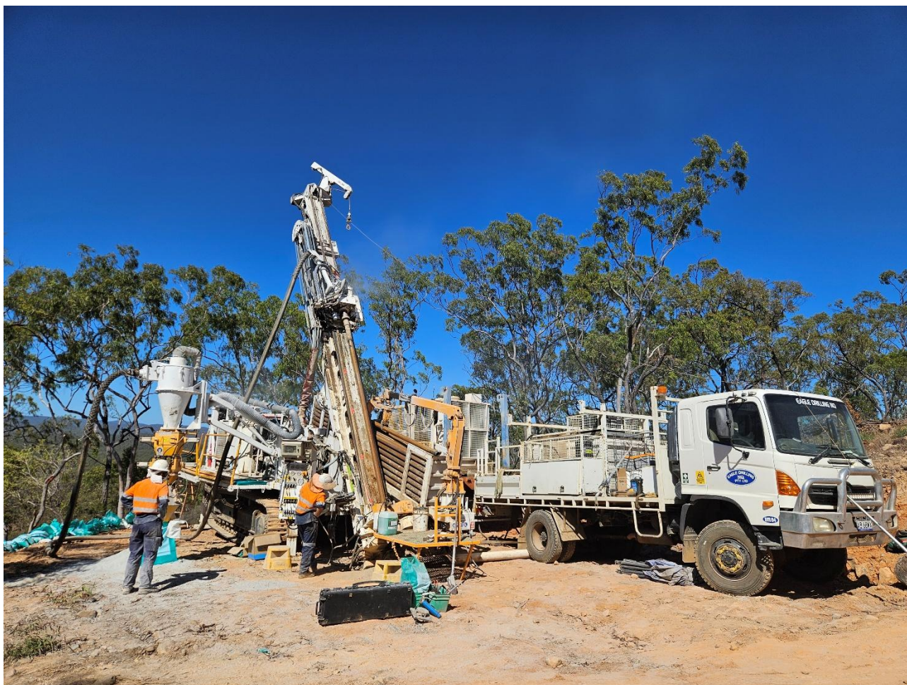
Figure 1 RC Drill Rig drilling ORR119
