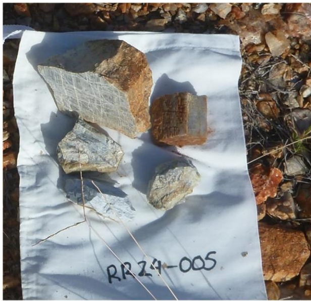
Figure 17. Rock chip samples of QXRD confirmed spodumene from the GMF Pegmatite.
