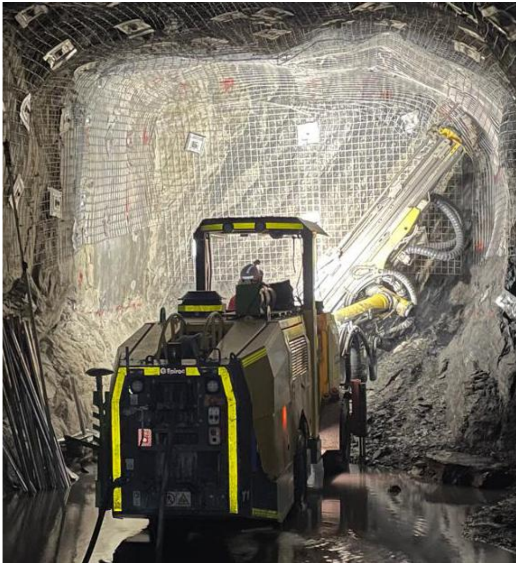
Figure 2 – Jumbo bolting drill cuddy on Lady Belmore Vein.
