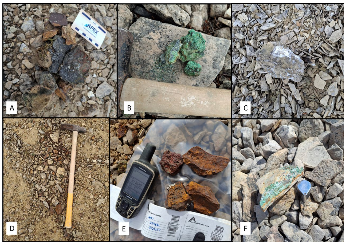
Figure 9: Examples of the interpreted copper gossans and outcrop from the Storm-Tornado area. For detailed descriptions of samples A-F above, see Table 4 in this report. Portable XRF was used to aid visual identification and these samples have not yet been analysed by laboratory.
