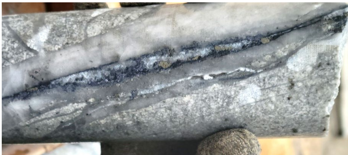
Figure 13: Photo of molybdenite + quartz + pyrite veining within quartz monzonite porphyry stock in drill hole WD22-04 (interval 640.66-642.18m downhole which returned 0.22% Mo). 1
