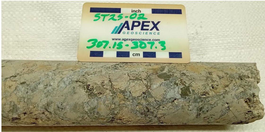
Figure 1: Dense breccia and fracture fill visual pyrite and chalcopyrite from ST25-02 (307.15-307.3m downhole). Assays for this interval are pending (see below visual estimates disclaimer).
