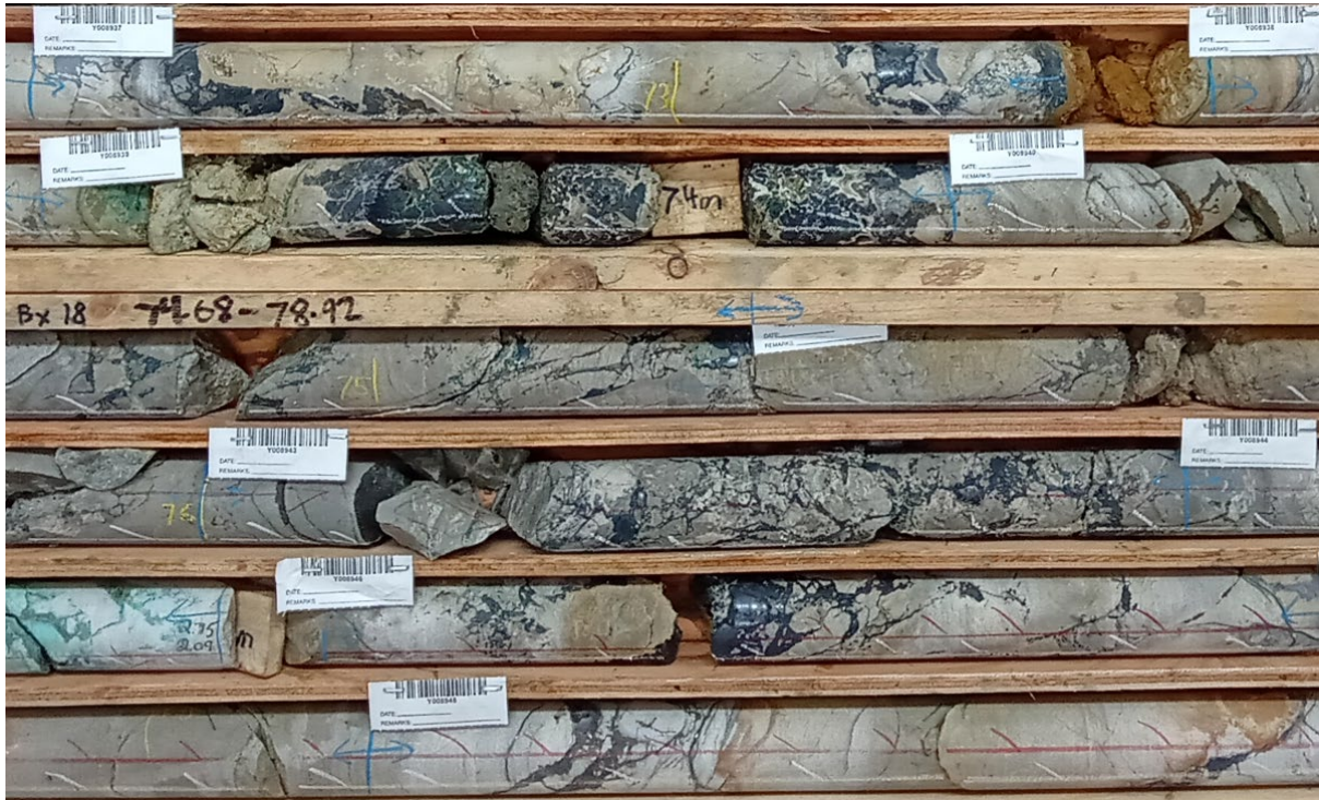
Figure 5: Dense semi-massive and breccia visual chalcocite (dark grey mineral) from PFS-002 (72.7-78.6m downhole). Assays for this interval are pending.
