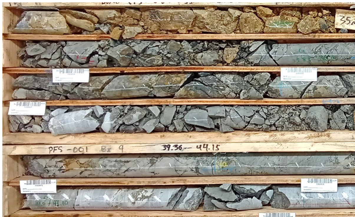
Figure 3: Dense breccia and semi-massive visual chalcocite (dark grey mineral) in drill hole PFS-001 (33.94-41.4m downhole). Assays for this interval are pending.
