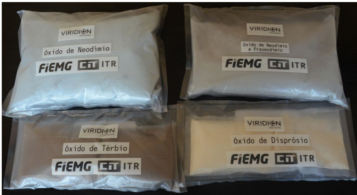
Figure 5: Recycled high-purity Nd, Pr, Dy, Tb oxides delivered to CIT SENAI ITR / FIEMG, originating from end-of-life magnets recovered in Brazil and processed at Ionic Technologies’ facility in Belfast, UK.
