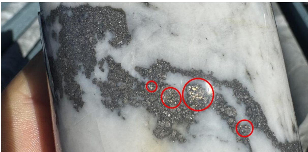
Figure 3. Diamond drill core from AMD003 at 180.0 metres down hole showing abundant grains of visible gold (yellow) hosted within an arsenopyrite vein (grey) in milky quartz. This interval graded 0.7 metres at 446g/t gold from 179.6m 2 .
