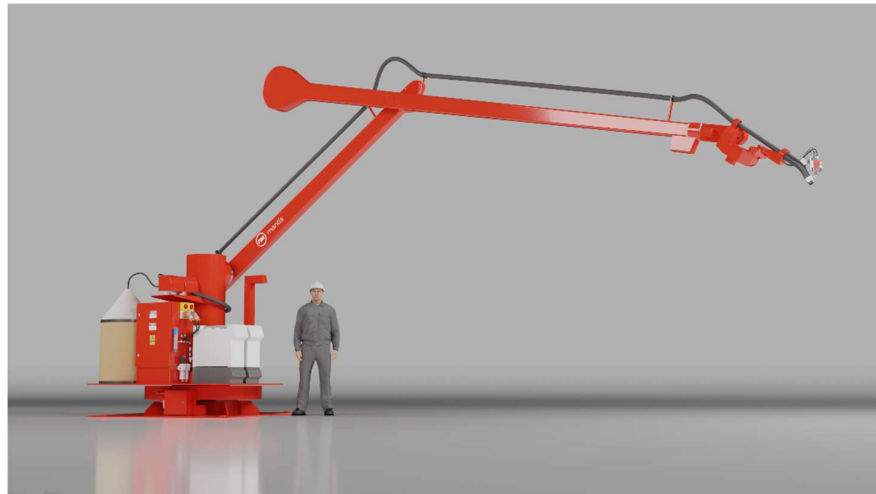
A render of the DST® enabled Mantis™ robot, highlighting its significant 8-metre reach
