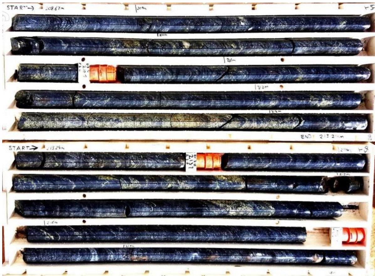
Hole 18CB054 intersection disseminated chalcopyrite-pyrite with accessory pyrrhotite in magnetite-chlorite quartz shear, 7m @ 1.97% Cu and 0.48 g/t Au from 208m downhole ( see assay table)
