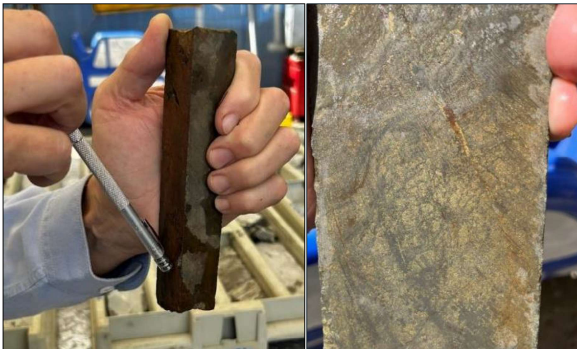
Figure 4: Photos of the highly magnetitic mineralised drill core (pyrrhotite) in diamond core hole CC0036D, responding strongly to a hand-held magnet.
