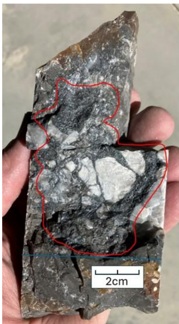
Figure 3 – MR103 stibnite filled quartz vein breccia at 198.9m
