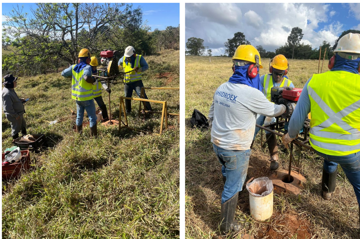
Figure 4 – Auger drilling underway at the Araxa Project.
