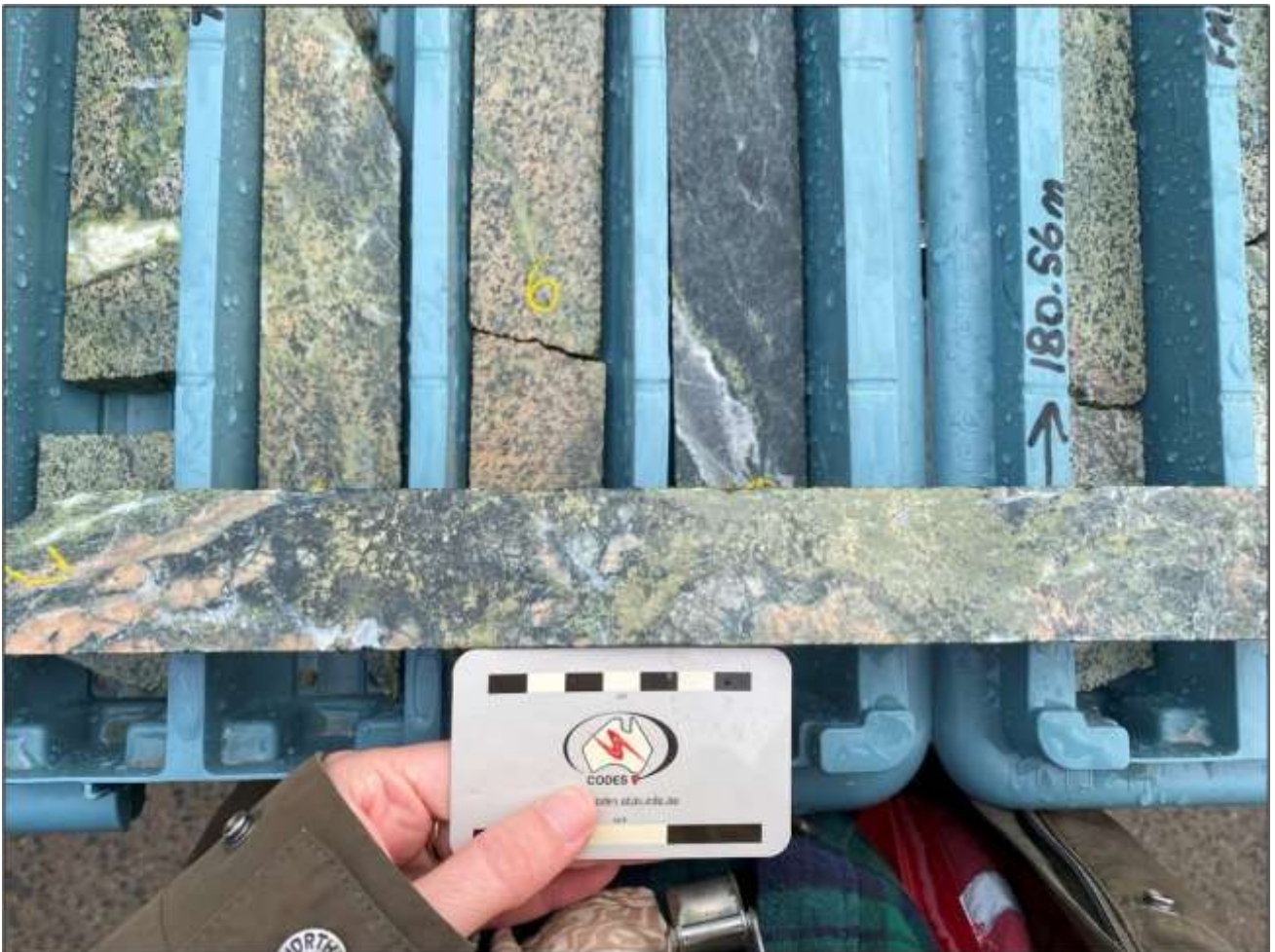
Figure 5. Intensely altered zone with epidote-secondary magnetite-quartz-k-feldspar-chlorite-actinolite-anhydrite with sulphides including chalcopyrite-pyrite-bornite-chalcocite-covellite (FMD0508, 178 m)
