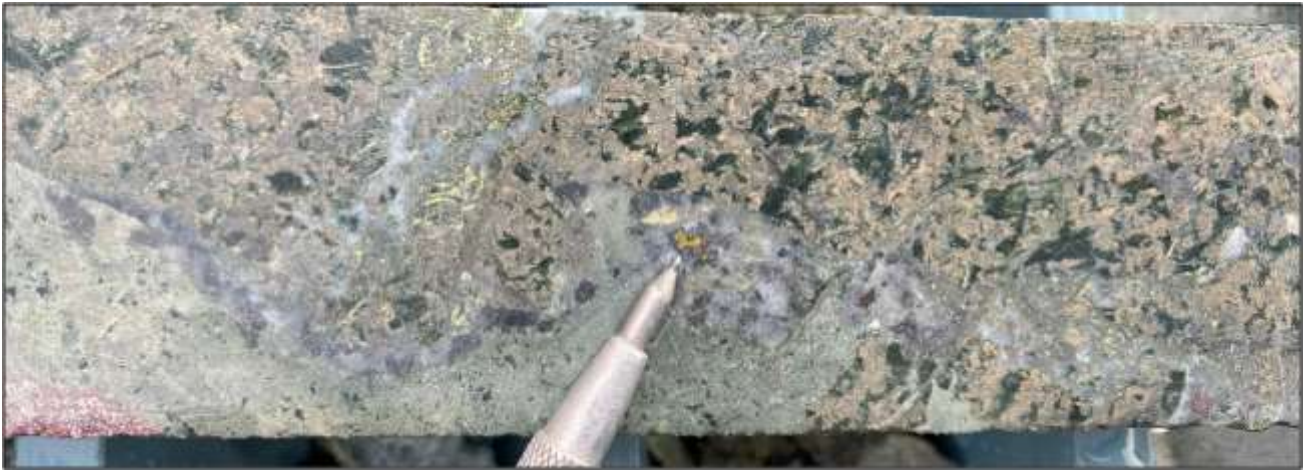
Figure 4. Quartz-molybdenite-chalcopyrite-bornite-chalcocite B vein (quartz-sulphide vein) within diorite-andesite host rock (FMD0508, 148 m, 0.15% Cu)
