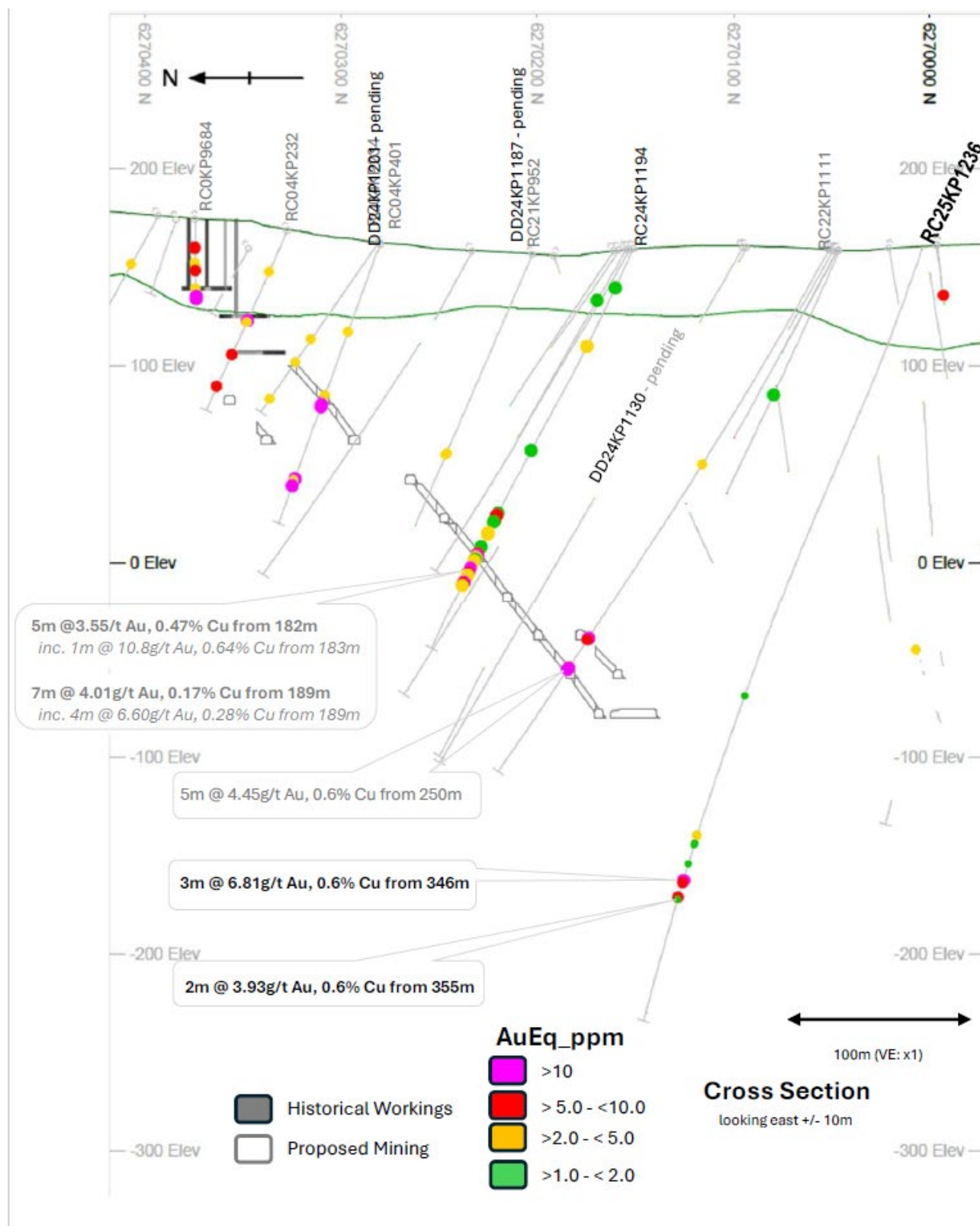
Figure 5: Cross section B-B' (refer Annexure 1 for section orientation) through the Hillsborough lodes with recent drilling results.
