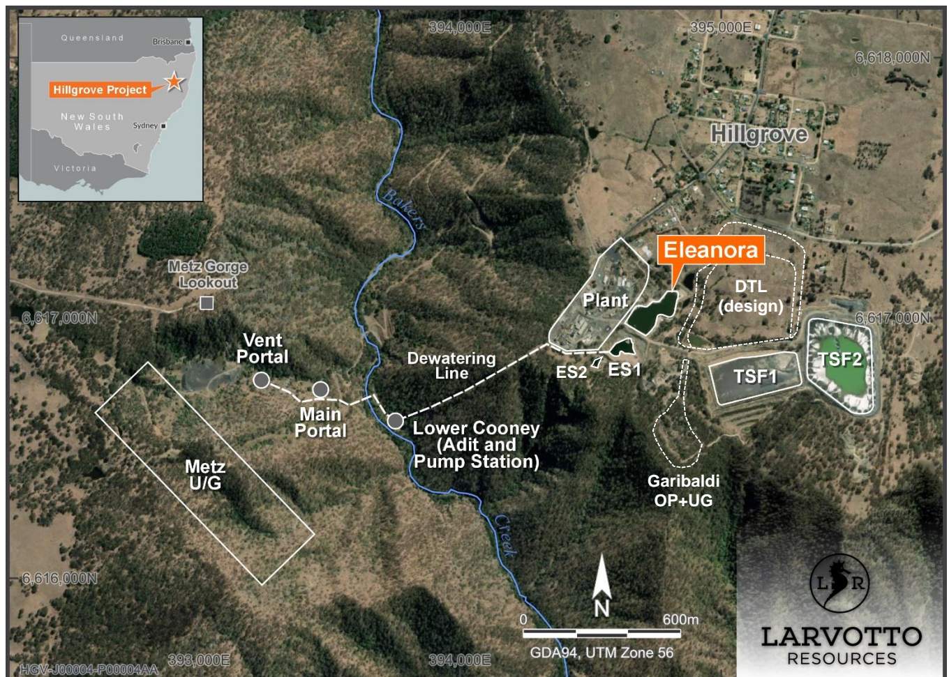
Figure 10 Water management infrastructure at Hillgrove Mine
