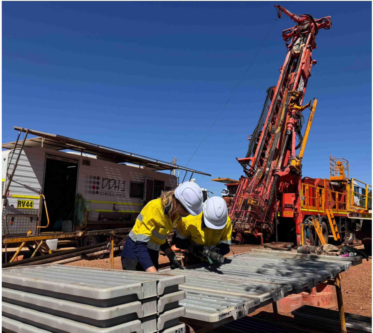
Photo 1. DDH1 truck-mounted diamond drill rig #46 on drill hole 25MYDD007 targeting mineralisation at Gossan Hill Prospect. Kairos Geologist Emilie Boulter (left) and Senior Geologist Will Coussens inspecting mineralisation at freshly drilled core.
