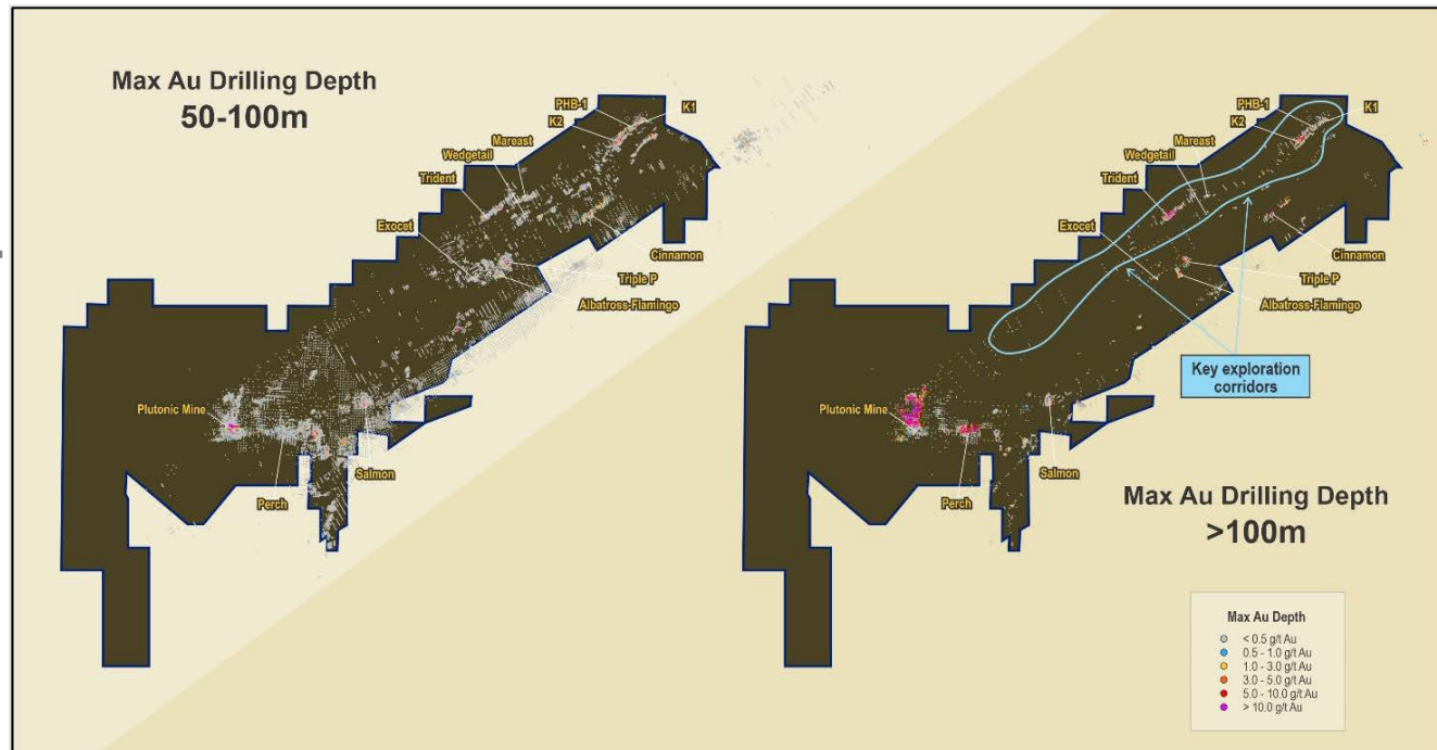
Figure 7: Plutonic gold belt showing mineralisation below 100m versus drilling density below 100m
