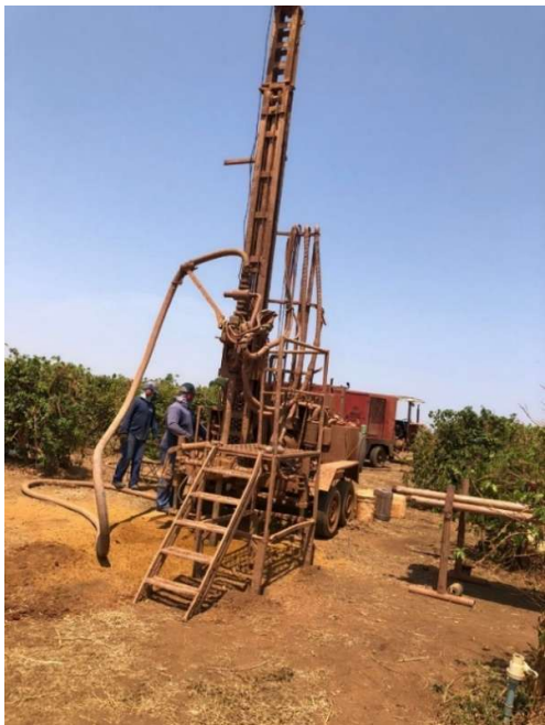
Figure 1: RC drill rig operating in the CODA Central project near the coffee plantation
