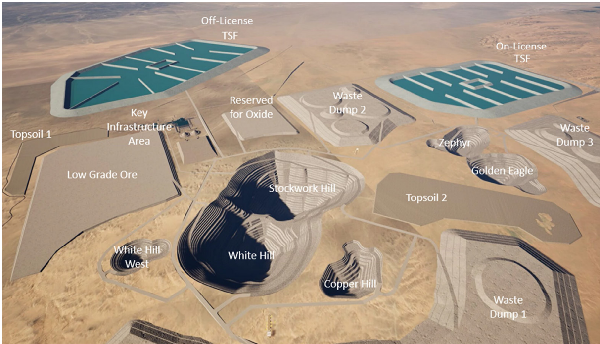
Figure 3: Kharmagtai PFS Site General Arrangement
