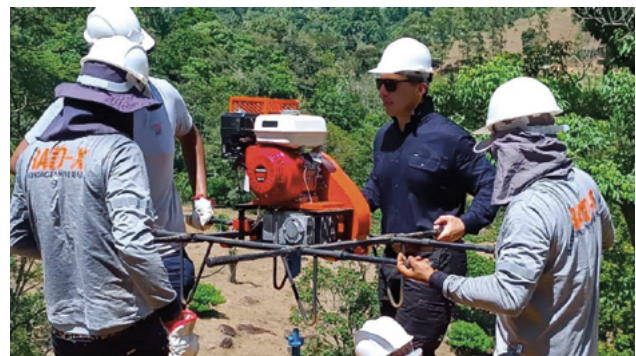
Auger drilling in the Rocha da Rocha Province.
