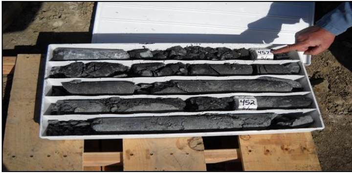
Figure 5: Drill cores showing metasomatic magnetite
