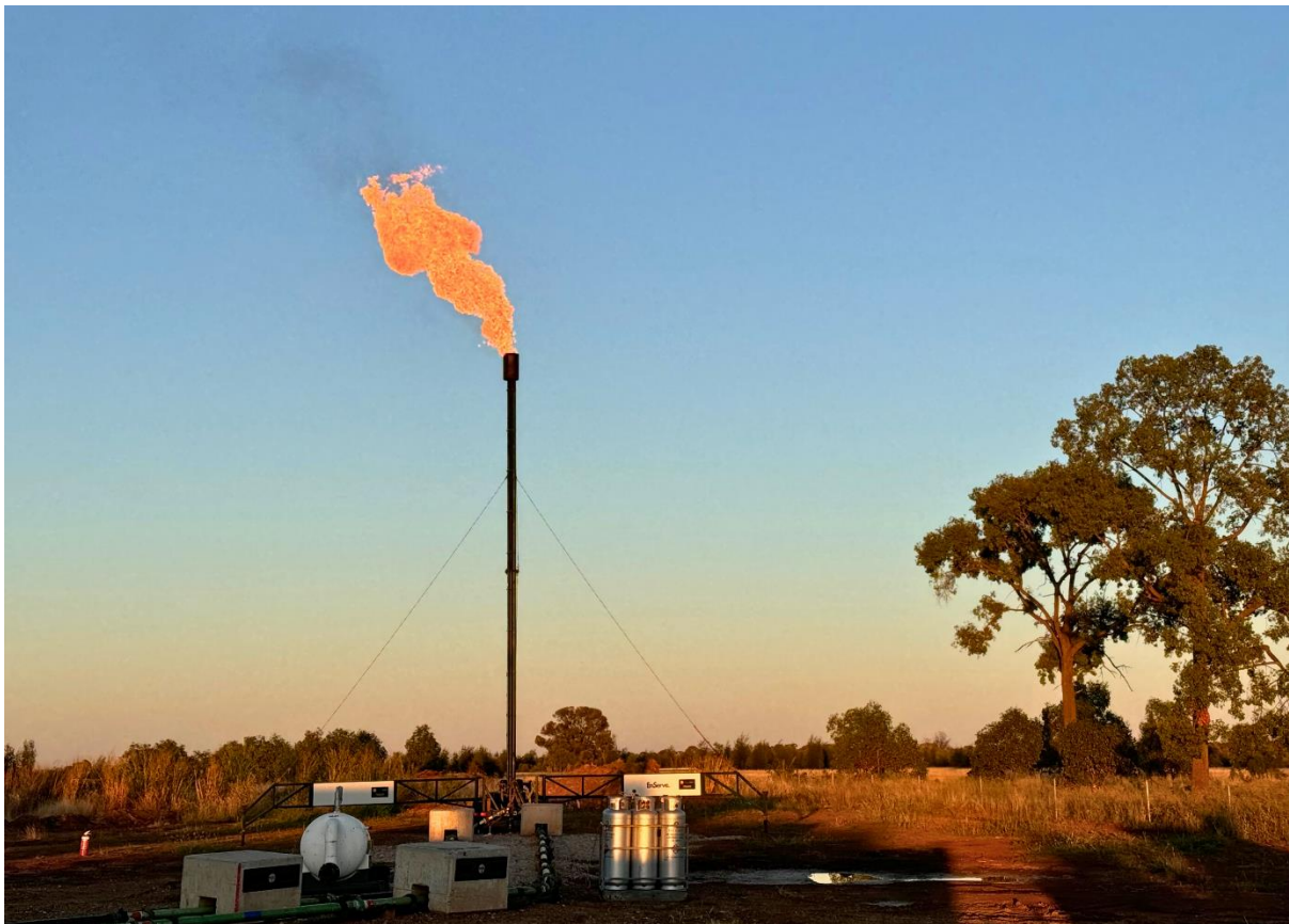
Figure 2: Flare while flow testing Canyon-1H well
