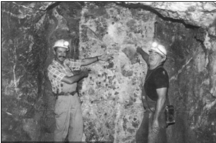
Figure 3 - Calcite-quartz breccia vein with 'wire silver' from 82m level. Clasts (100-350mm) in the breccia are mostly pyroxenite/peridotite, Elizabeth Hill mine 7 .
