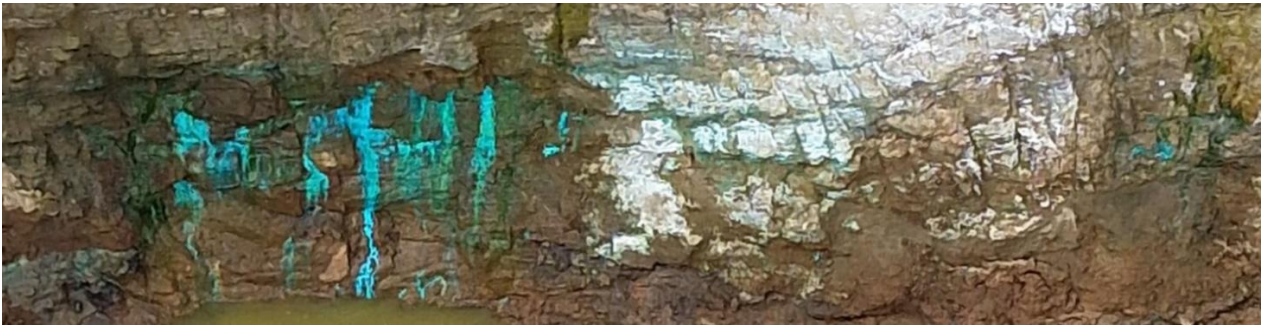
Copper and cobalt staining in the walls of the artisanal workings
