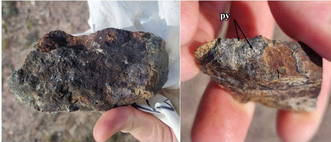
Figure 7: (Top Left): Gyrfalcon Prospect - Field photograph of LHNS05 (1.2% U_3O_8 ) – Chlorite-altered mafic rock with suspected fine disseminated black pitchblende (Top Right): Gyrfalcon Prospect - Field photograph of LHNS04 (0.57% U_3O_8 , 1.0% Mo) – Mafic rock with visible pyrite sulphide (py).
