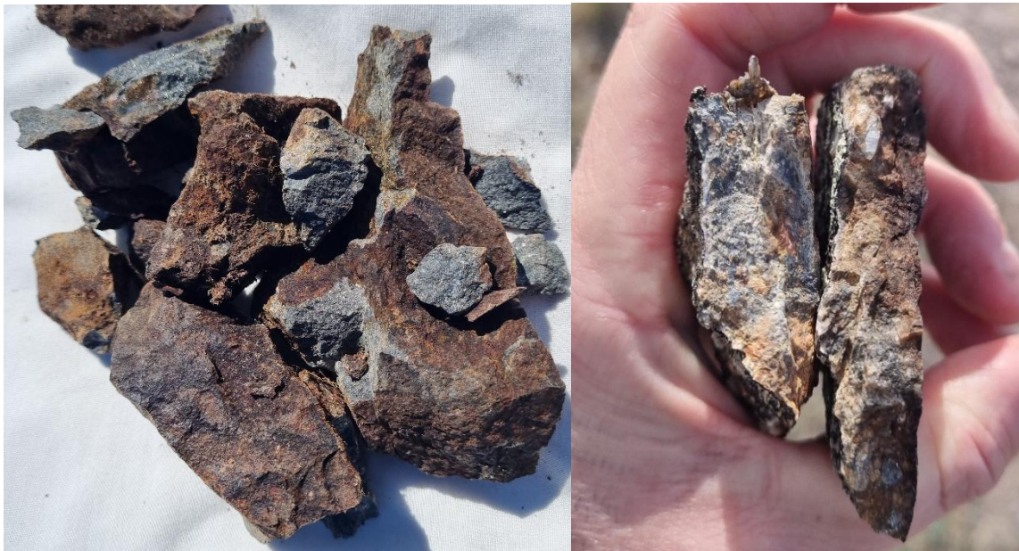
Figure 8: (Top Left): Snow Goose Prospect – Field photograph of LHNS07 (1.1% U_3O_8 , 0.34% Mo) – Altered mafic rock with disseminated pyrite (Top Right): Snow Goose Prospect – Field photograph of KHNLO2 (0.29% U_3O_8 ) – Felsic intrusive rocks.
