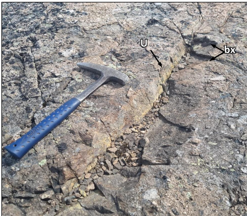
Figure 9: Field photograph of the altered and brecciated mafic outcrop with a yellowish uranophane-bearing (U) fracture, from which sample LHNS13 was collected. This sample returned up to 0.3% U_3O_8 and 0.13% Mo from the Tundra Swan prospect. Note the presence of breccia clast fragments (bx).
