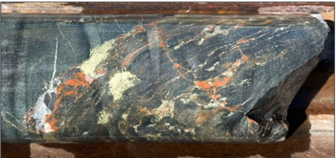
Figure 6. RMD001 showing a shear zone with magnetite, biotite, red rock, chalcopyrite and pyrite, at 306m down hole.
