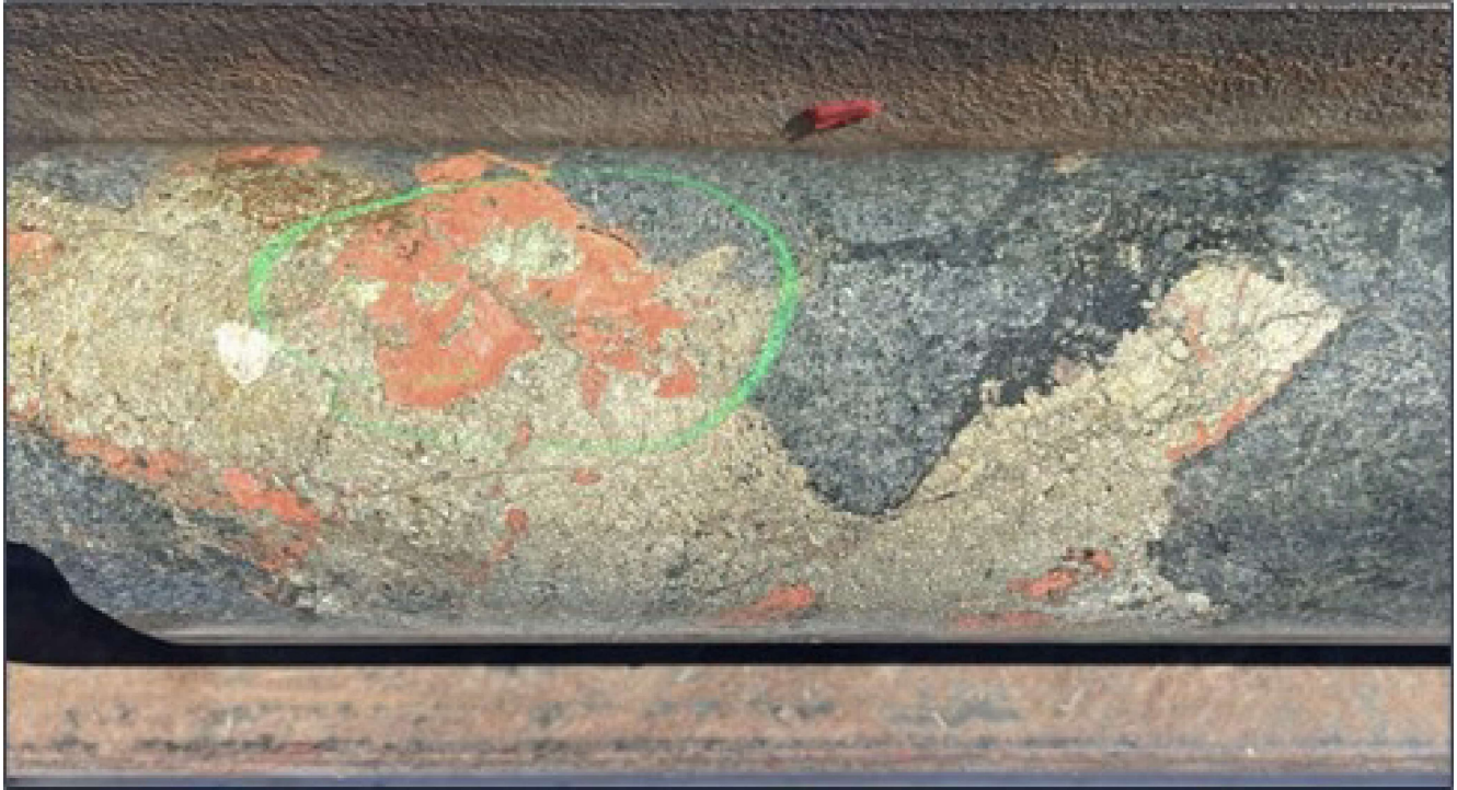
Figure 7. RMD001 breccia zone showing massive pyrite, red rock and chalcopyrite, at 532.5m down hole
