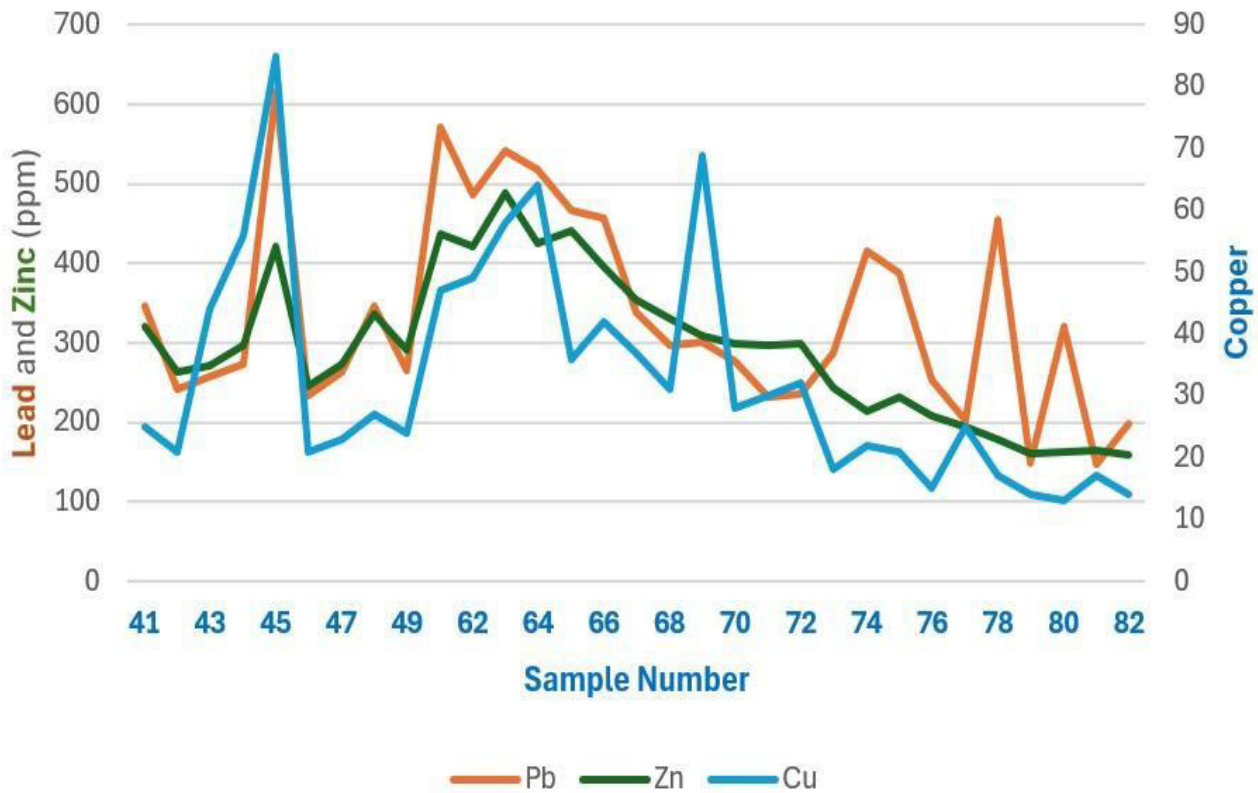
Figure 7. Chart of copper, lead and zinc values in parts per million (ppm) in the anomalous gold samples.
