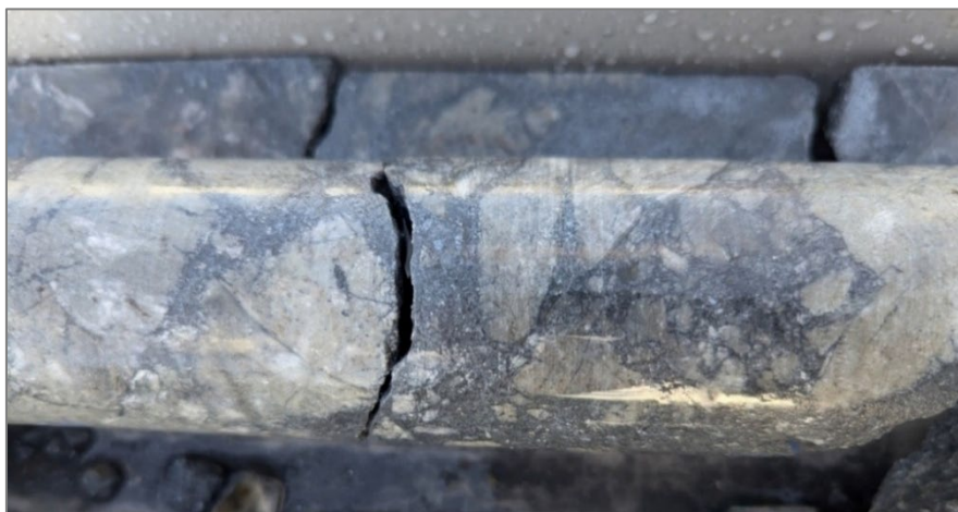
Figure 16: Core photo of the high-grade Sb interval in RDRC067 highlighting brecciated ultramafic at 239.4m. Refer ASX Release 26 August for full context)
