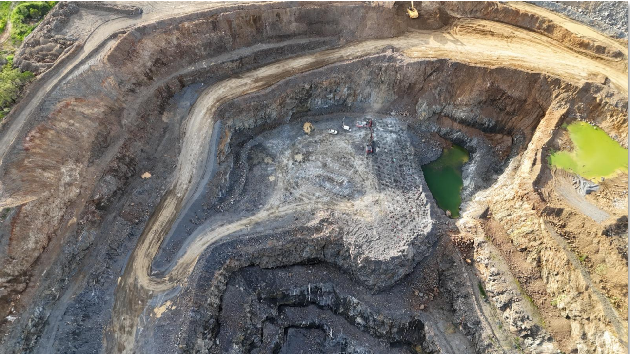
Pictured: The Southeast corner of the Open Pit, initial focus of the Stage II pit stripping and cut back with the Iolanthe and Bluff vein package as main targets with drilling progressing at 345-335 RL.
