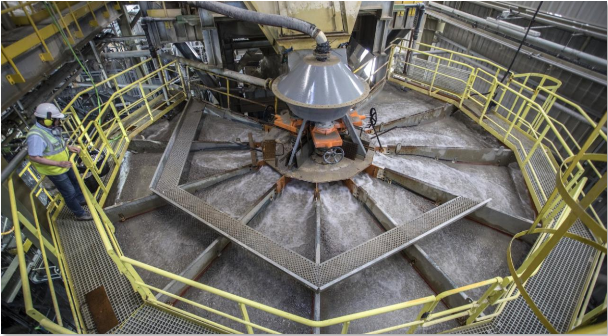
Pictured: Monitoring the Mineral Jigs at the Gravity Plant at Saloro.
