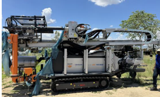
Figure 3. New Sonic drill rig with capacity to convert to Diamond drilling
