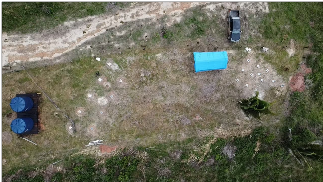
Figure 18. Ema permeability field trial setup. White squares are the concreted collars of the drill holes which will be injected with water and/or lixiviant pumped from the blue storage tanks. Two separate test zones have been developed, one with shallow holes drilled to 5.7m depth (adjacent to car) and test zone 2 with both injection and extraction holes drilled to 10m depth adjacent to the 2 10,000 litre water storage tanks.
