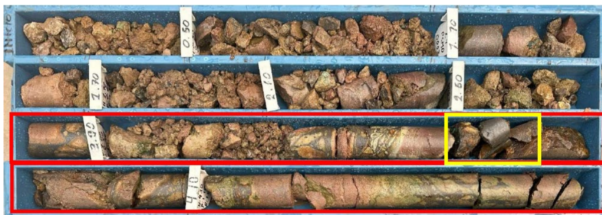
Figure 3: PCHA PROJECT – HIGH-GRADE COPPER-SILVER MINERALISATION AT COBREMANI TARGET
