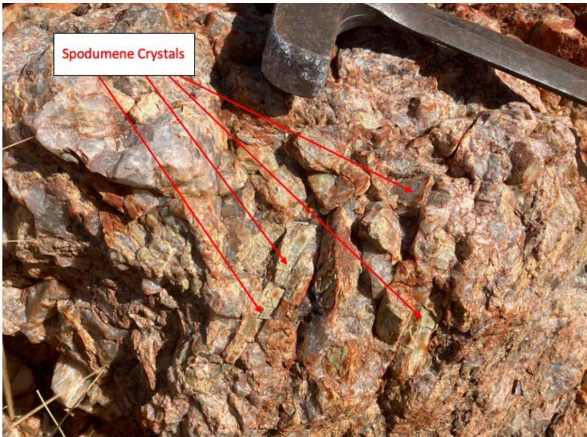
Figure 6. Spodumene crystals seen in outcrop at the Mt Marie lithium prospect
