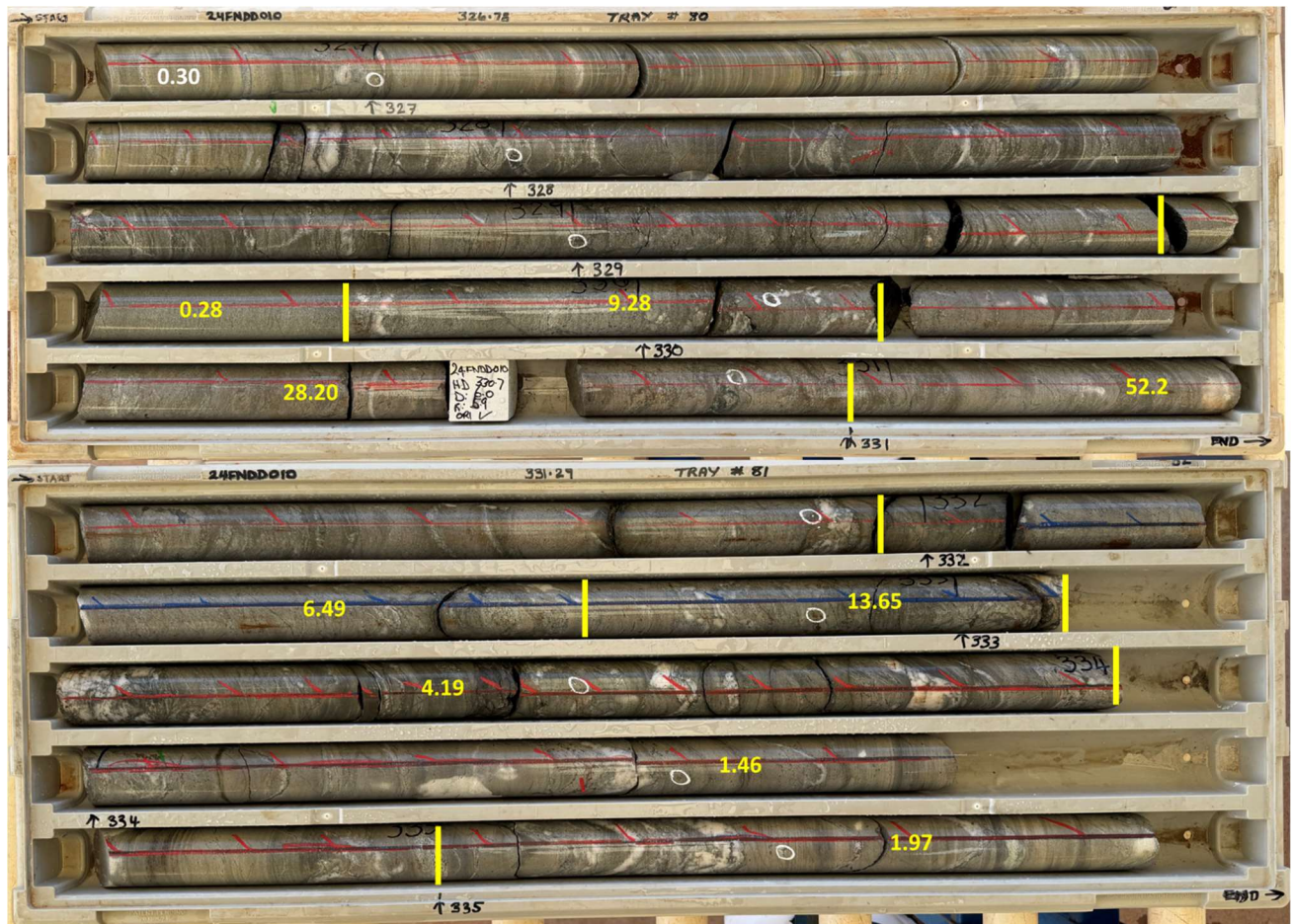
Plate 2 :24FNDD010 drill core from 326.78m to 335.6m with gold values (g/t) annotated in yellow
