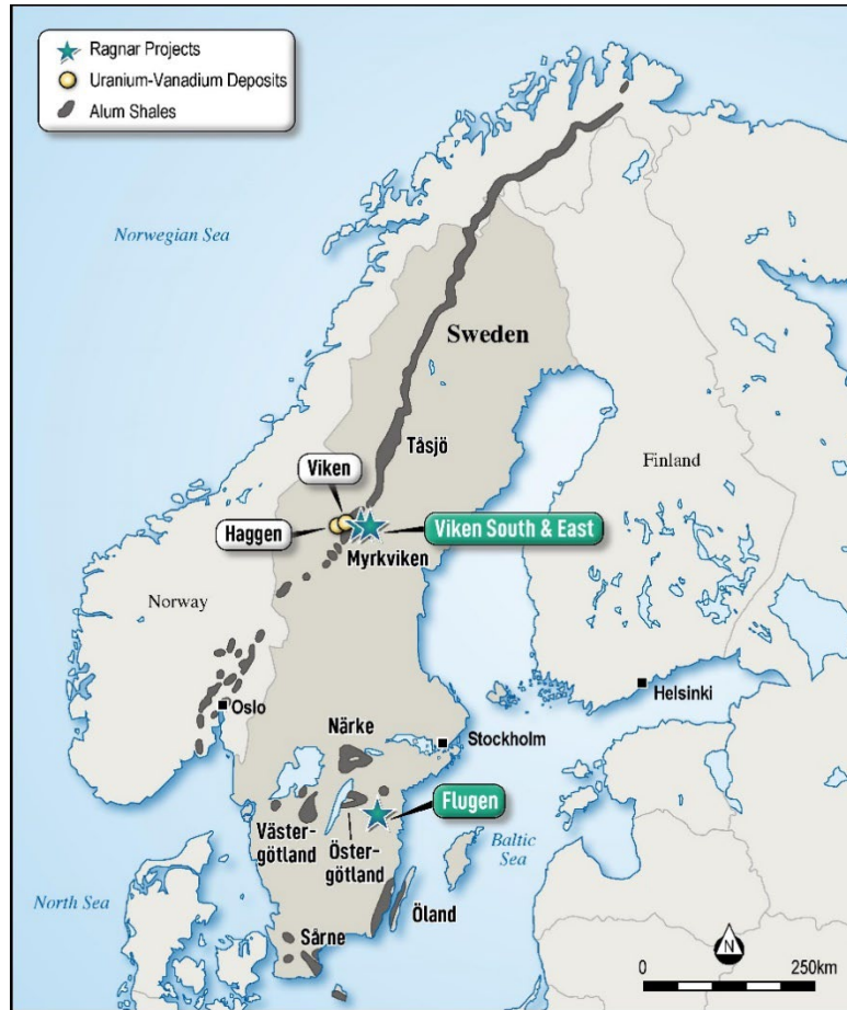
Figure 6: Map of Scandinavia showing the distribution of alum shales (black), which are the primary host rock for uranium mineralisation in Sweden, and the location of Ragnar's energy metals projects (green) in relation to nearby uranium-vanadium deposits 2
